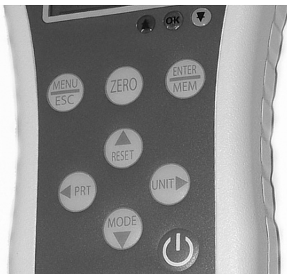
Figure 1 GTX Plus control panel
