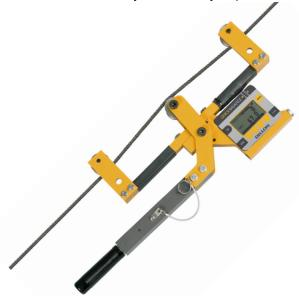
Figure 3.2 Quick Balance attached to cable
