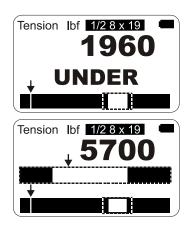
Figure 3.4 Check-tension display
