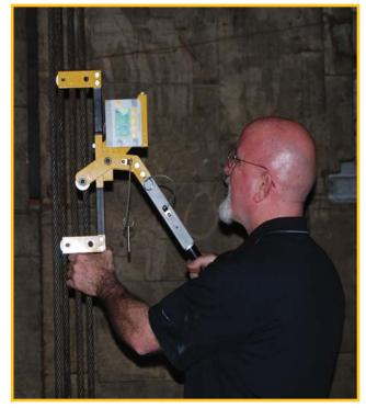
To test wire rope tension using standard equipment, it would take a service technician approximately one hour to tension the wire ropes with a spring-type scale, requiring a "trial-and-error" process to ensure each was tensioned equally. For elevator modifications, the process became more complex, as MEI personnel needed to weigh the elevator car before and after modifications took place to ensure the elevator still bore a suitable load—defined as no more than a 5 percent increase in gross load.
