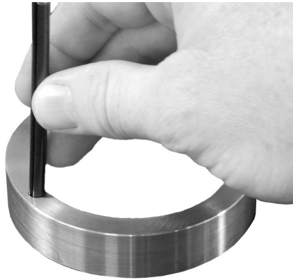
Figure 5.2 Inserting Roll Pin
