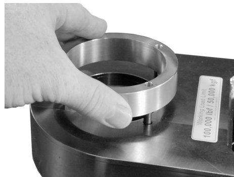
Figure 5.4 Placing Second Spacer on Roll Pins
