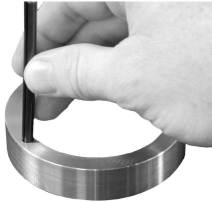
Figure 5.2 Inserting Roll Pin
