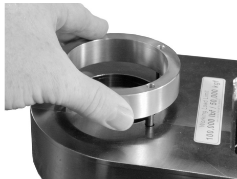
Figure 5.4 Placing Second Spacer on Roll Pins
